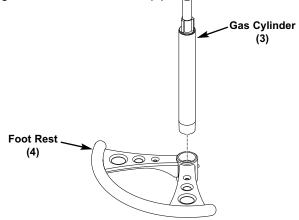
3. Press the bottom of the Gas Cylinder into the center hole of the Base Assembly.
